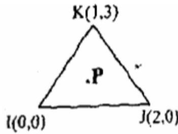
6. Calculate the element stiffness matrix and thermal force vector for the plane stress element shown in fig. The element experiences a rise of  $10^\circ\text{C}$
