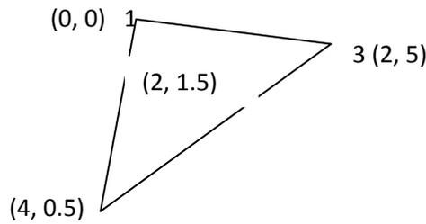
5. Find the temperature at point (1, 1.5) inside a triangular element shown with nodal temperature given as  $T_i = 40^\circ\text{C}$ ,  $T_j = 34^\circ\text{C}$  and  $T_k = 46^\circ\text{C}$ . Also Calculate the location of the  $42^\circ\text{C}$  contour line for triangular element shown in fig.
