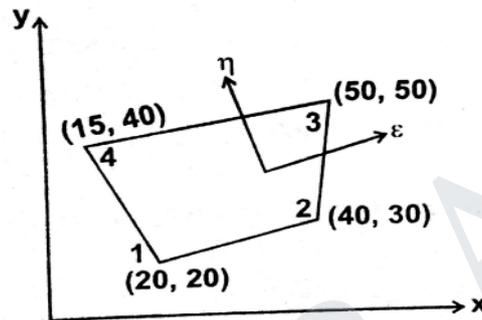
5. Evaluate the Jacobian matrix at the local coordinates  $\epsilon = \eta = 0.5$  for the linear quadrilateral element with its global coordinates as shown in fig. Also evaluate the strain-displacement matrix.
