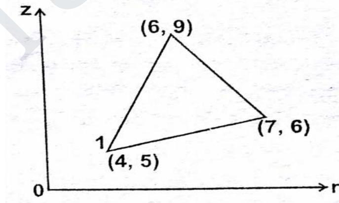
8. For an axisymmetric triangular elements as shown in fig. Evaluate the stiffness matrix. Take modulus of elasticity  $E = 210 \text{ GPa}$ . Poisson's ratio = 0.25. the coordinates are given in millimetres.
