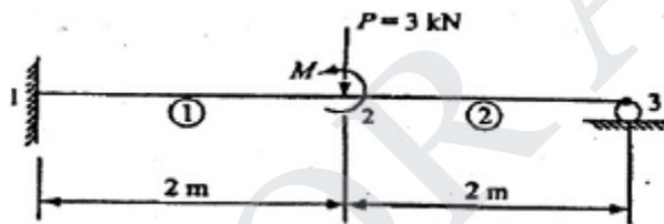
9. For the beam and loading as shown in figure. Calculate the slopes at nodes 2 and 3 and the vertical deflection at the mid-point of the distributed load. Take  $E=200 \text{ GPa}$  and  $I=4 \times 10^{-6} \text{ m}^4$
