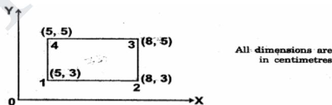
8. A 3 noded triangular element as shown in fig Calculate the temperature at the point P (4, 3), given that the temperatures at nodes 1, 2 and 3 are 75°C, 90°C and 60°C respectively.
