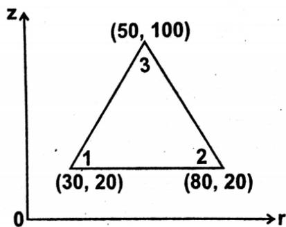
9. The nodal coordinates for an axisymmetric triangular element shown in fig are given below. Calculate the strain-displacement matrix for that element
