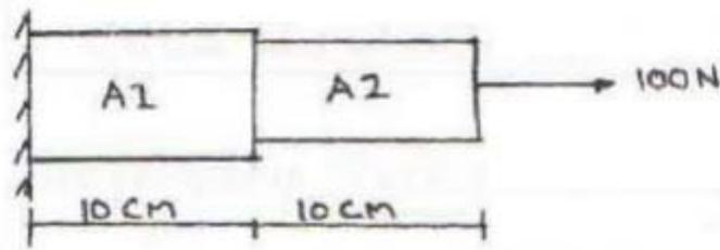
3. Consider the bar shown in figure axial force  $P = 30\text{KN}$  is applied as shown. Determine the nodal displacement, stresses in each element and reaction forces.
