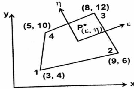
4. For the four noded quadrilateral element shown in fig determine the Jacobian and evaluate its value at the point  $(1/2, 1/2)$
